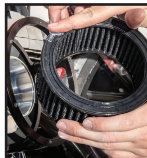
Install filter gasket ring into cage. Lube both filter bases with O-ring lube and install into cage
