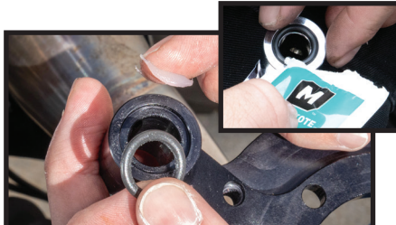
Lube and install inner and outer breather O-rings, use with O-ring lube.
