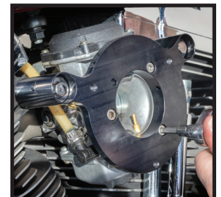
Insert backing plate bolts to help center backing plate & breather bolt holes. Final torque breather bolts to 22-24 ft/lbs. Final torque backing plate bolts to 36-60 in/lbs (Carburetor) 72 in/lbs (EFI) models.
