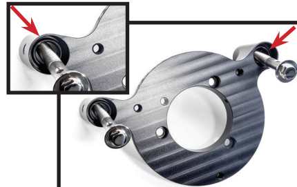
Install breather bolts with outer breather O-rings
