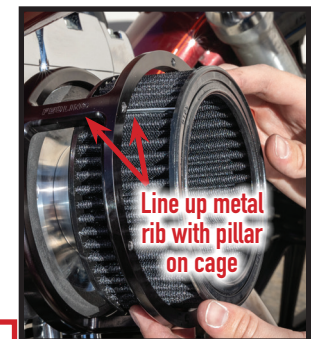
Alternately tighten velocity stack bolts. Final torque to 72 in/lbs.
