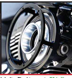
Alternately tighten velocity stack bolts. Final torque to 72 in/lbs.
