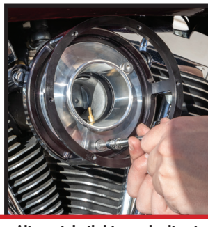
Alternately tighten velocity stack bolts. Final torque to 72 in/lbs.
