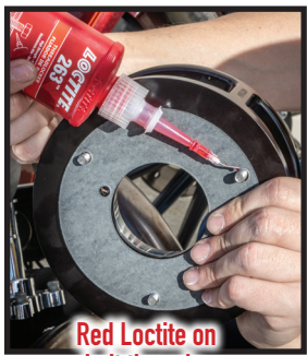
Install velocity stack, gaskets and bolts.
