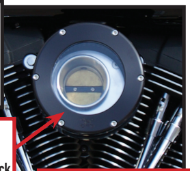
Install cover with logo at the six o'clock position
