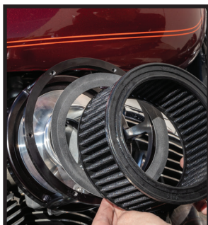
Install filter gasket ring into cage. Lube both filter bases with O-ring lube and install into cage
