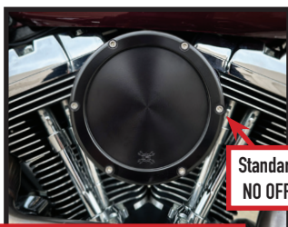
Install cover with logo at the six o'clock position
