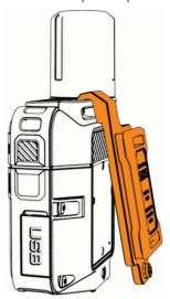
2 Using a T10 TORX screwdriver, secure the spine mount adapter over the back of the device using the screw included with the adapter.
