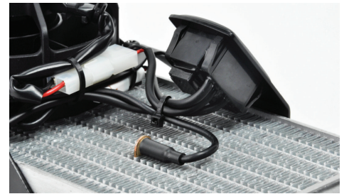
Sensor Installed (Clean, No Grease/Damage)
