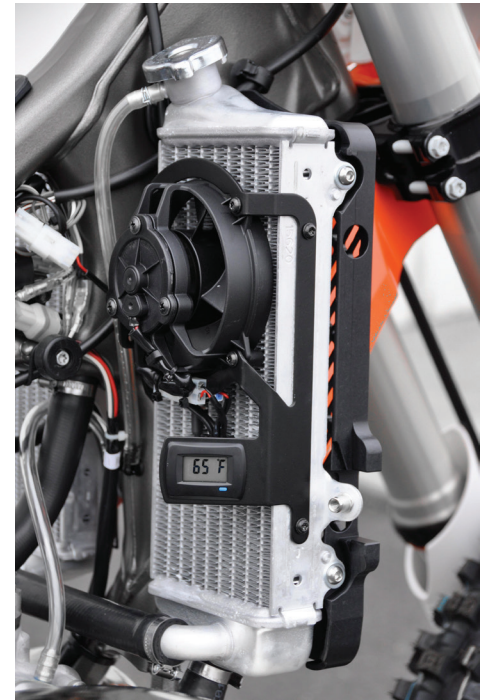
Fan Kit Installed (Varies by Model)
