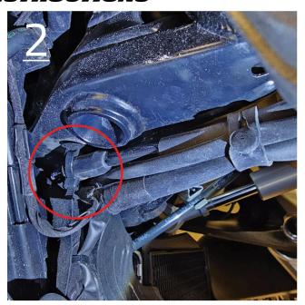
On the right side. Cut the zip tie holding the brake line. Seperate brake line from other lines and install a new zip tie on rubber grommet as shown in figure 2.
