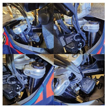
Make sure all cables and line have the necessary slack in them after the risers are installed. When routed properly the cables and lines should not be tight when turned side to side. They may come in contact with the triple clamp some, that will be ok. Also be sure that the cables do not get pinched between the triple clamp and steering lock stop.
