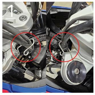
Remove both line loops from the triple clamp.
