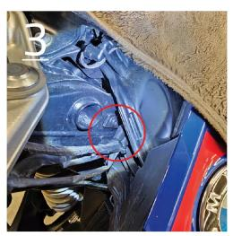
On the left side, cut the cable tie holding the lines to the frame as shown in figure 3. You will use a new cable tie around the wires to hold them together without connecting them back to the frame so they will have more mobility.
