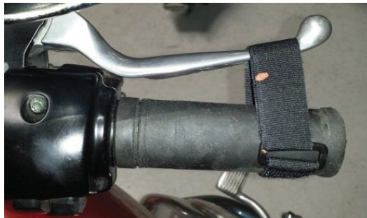
Brake Lever Strap: for use as a parking brake.
