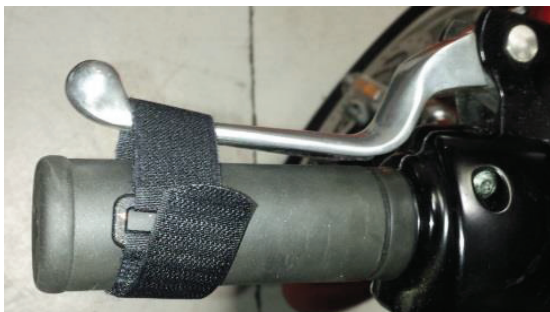
Clutch Lever Strap: to prevent unwanted launching.
