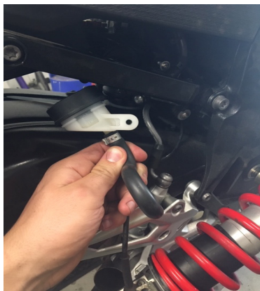
Remove original reservoir
