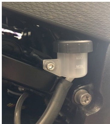
Install new reservoir offset from original position using spacer & bolt provided
