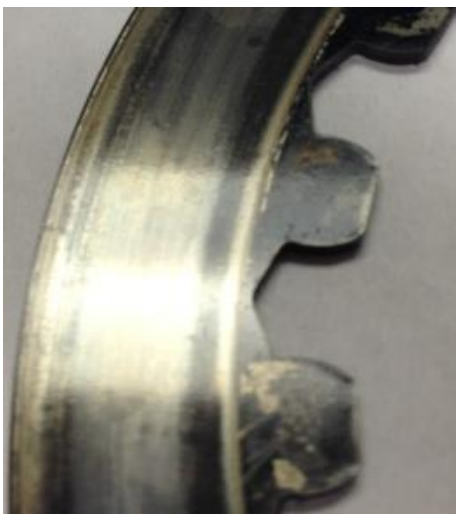
Excessive Heat (Black)
