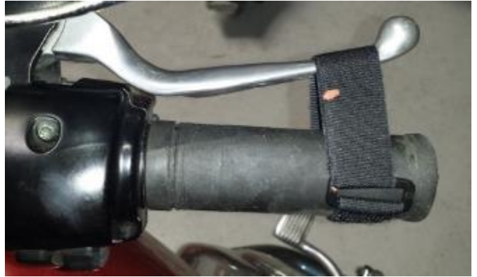
Brake lever strap: Use as a parking brake.
