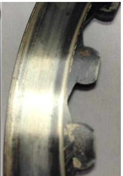
Excessive Heat (Black)
