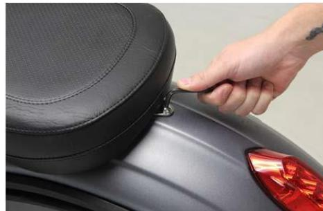
4. Secure seat to fender using supplied 8mm x 15mm buttonhead Allen screw. Tighten securely with a 5mm Allen wrench.
