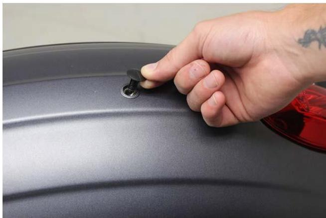
3. Engage the Mustang seat's front bracket with the shoulder screw and lower the seat to the fender
