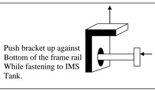
Be sure that the tank is mounted securely and does not bind or in any way inhibit the controls or function of the vehicle. Ensure that there are no sharp objects that rub against the tank which may eventually puncture the tank. Fill the fuel tank and install IMS gas cap. CHECK FOR ANY LEAKS. NO LEAKS. ENJOY YOUR RIDE!!
