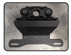
2. Install (No. 1) 13710-FEBKT-1, fender eliminator bracket to stock rear fender reinforcement bracket using (No. 8) M6X14BHS, 6mm screws.
