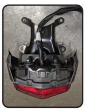
4. Install (No. 3) 070BG-LH-K1, led light onto (No. 1) 13710-FEBKT-1, fender eliminator bracket using (No. 10). M4X6BHS, 4mm screws.
