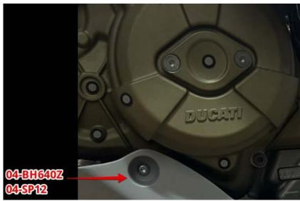
3- **IMPORTANT** -Secure all bolts with BLUE LOCTITE during final assembly.
