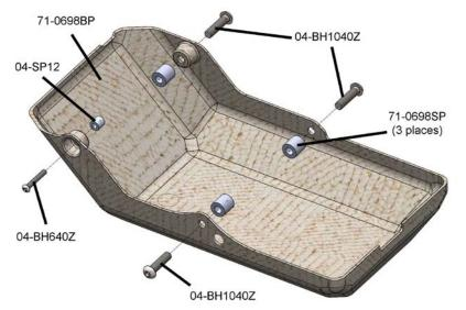
2- On the LHS forward most location, remove the OEM engine case bolt (photo to right) and replace with the supplied 04-BH640Z bolt and 04-SP12 spacer.
