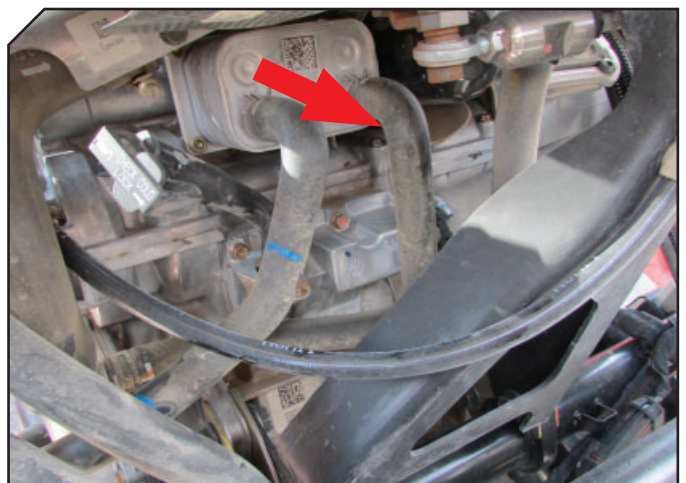
REMOVE STOCK COOLANT LINE
