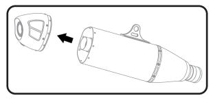
4. Remove baffle and clean carbon buildup. Inspect stainless steel mesh wrap on baffle.
