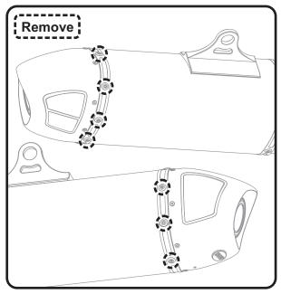
3. Carefully remove endcap assembly by pulling outward and remove old packing.
