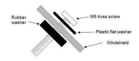
Again, do not overtighten, it isn't necessary and can damage the well nuts.
