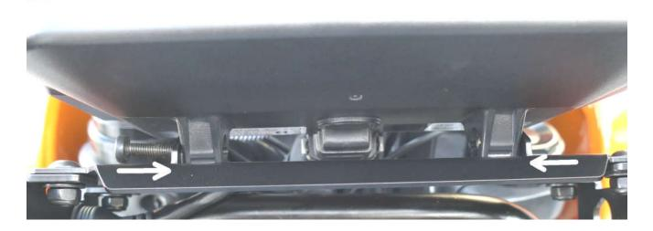
Insert the M5 x 35 Phillips screws in each side and screw them in until snug. Take care not to push hard on the screwdriver, you could push the well nut out of the other side.
