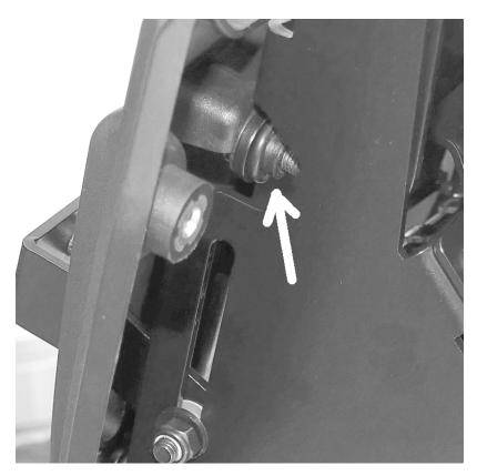
Insert one rubber well nut on each side of the display from the outside (see photo below).
