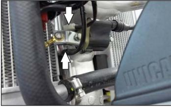
11 Unplug both of the stock coil wires.
