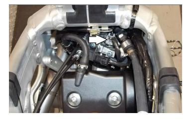
5 Unplug the stock Fuel Injector at the top of the throttle body.
