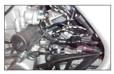
10 Plug the PC6 wiring harness in-line of the stock Crank Position Sensor connectors.
