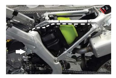
4 Remove the left engine mount on the left side of the cylinder head to aid in routing of the harness to the TPS and Crank Position Sensor.
