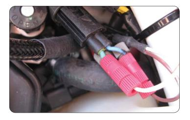
7 Use the 2 supplied Positaps to attach the crank input wires of the PC6 to the stock crank position sensor wires.
