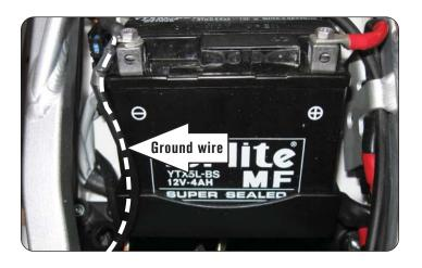
4 Attach the ground wire from the PC6 to the negative side of the battery.
