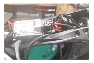
A Route the PC6 wiring harness up towards the battery and the top of the sub frame staying inside the frame rails as shown.
