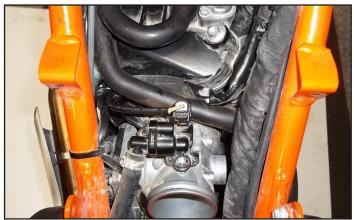
12 Plug the PC6 in-line of the stock injector and wiring harness.
