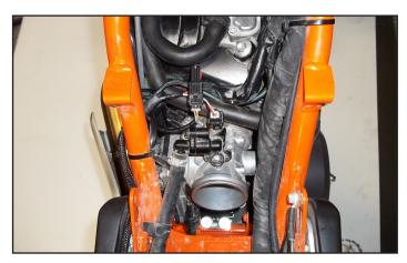
13 On the right side of the engine, locate and unplug the stock BLACK 2-pin connector from the inner coil stick and the stock WHITE 2-pin connector from the outer coil stick.
