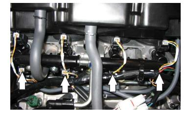
6 Unplug the stock wiring harness from the LOWER injectors.
