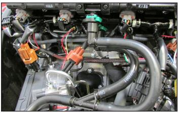
6 Plug the PC6 harness in-line of the stock wiring harness and injectors.
