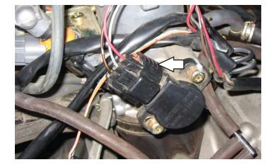
8 Unplug the stock wiring harness from the Throttle Position Sensor.
