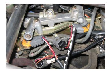
7 Plug the connectors from the PC6 in-line of the stock wiring harness and the Fuel Injectors.
