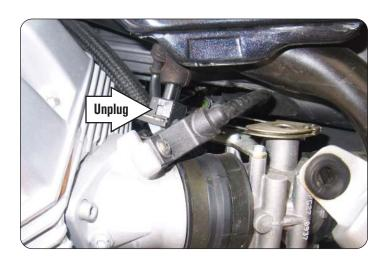
5 Unplug the stock wiring harness from the fuel injector on the LEFT cylinder head.
