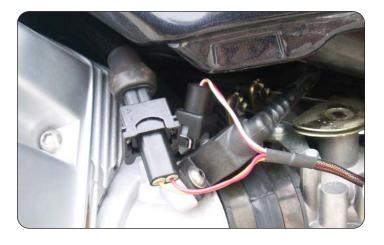
6 Plug the pair of PC6 leads with ORANGE colored wires in-line of the LEFT cylinder fuel injector and the stock wiring harness.
