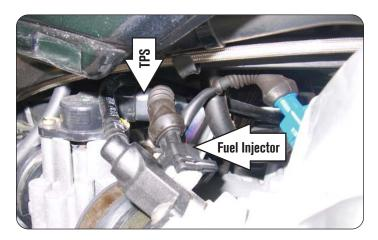
9 Using the supplied Positap, attach the GREY wire of the PC6 to the stock RED wire of the TPS wiring harness.
