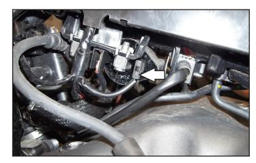
Plug the pair of PC6 wires with spade connectors (BLUE and WHITE/BLUE wires) in-line of the right cylinder ignition coil and the stock GREEN/RED wire.
