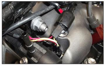
16 Plug the pair of PC6 connectors with YELLOW colored wires in-line of the right fuel injector and the stock connector.
