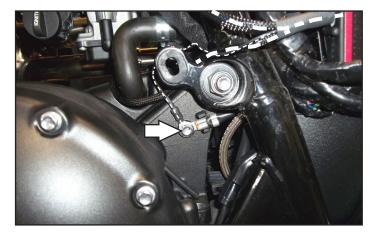
9 Unplug the throttle body servo connector on the right side of the bike.
