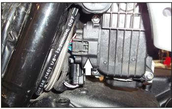
10 Plug the PC6 wiring harness in-line of the throttle body servo and stock wiring harness.
