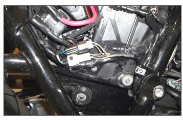
12 Plug the PC6 wiring harness in-line of the stock crank position sensor connectors.
