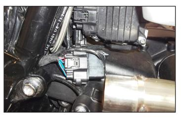
11 Unplug the crank position sensor connectors on the right side of the bike.
