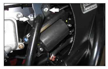
13 Remove the two bolts securing the coil bracket to the frame.
