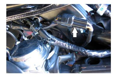
5 Unplug the BLACK 3-pin connector for the bike's Fuel Injectors on the left side of the frame behind and above the left throttle body.
