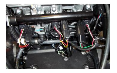
8 Plug the PC6 in-line of the stock harness and injectors.
