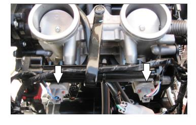
5 Unplug the stock wiring harness from the fuel injectors.
