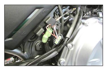
10 Plug the PC6 connectors in-line of the stock Crank Position Sensor connectors.
