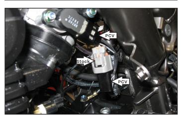
9 Locate and unplug the bike's Crank Position Sensor connectors on the right-hand side of the bike.
