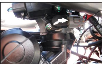
8 Plug the PC6 wiring harness in-line of the stock wiring harness and the TPS.
