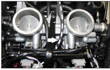
11 Route the remainder of the PC6 wiring harness with the coil connectors under the fuel rail, in between the throttle bodies, and up towards the coil sticks.
