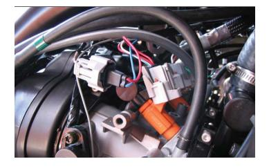
5 Plug the PC6 wiring harness in-line of the stock harness and the fuel injectors.
