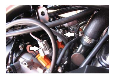
4 Unplug the stock wiring harness from each of the 4 fuel injectors.
