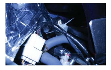
7 Plug the connectors from the PC6 in-line of the stock wiring harness and throttle bodies.
