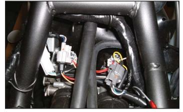
9 Locate the Throttle Position Sensor on the right hand side of the throttle bodies. This is the GREY 3-pin connector
