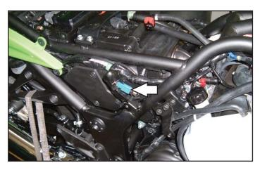
13 Unplug the Crank Position Sensor from the stock wiring harness.
