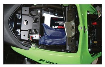
15 Using the supplied velcro, secure the PC6 unit in the tail section.
