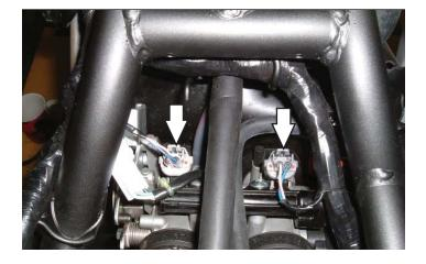
7 Unplug the stock wiring harness from each injector.
