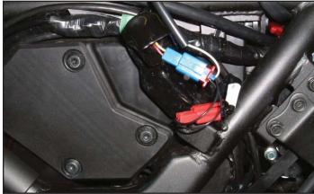
14 Plug the PC6 in-line of the stock wiring harness and CPS.
