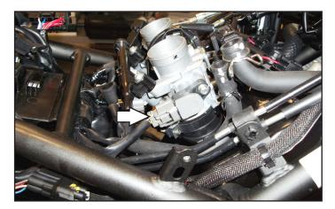
Plug the connectors from the PC6 wiring harness inline of the TPS and the stock wiring harness.
