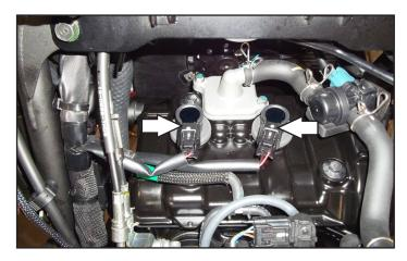
11 At the top of the engine, unplug the stock wiring harness from both of the Ignition Coils.
