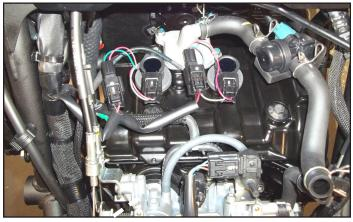
12 Plug the PC6 wiring harness in-line of the stock wiring harness and the Ignition Coils.
