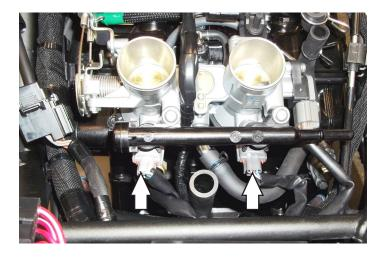
4 Unplug the stock wiring harness from both Fuel Injectors.
