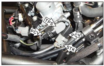
9 Locate and unplug the stock Crank Position Sensor connectors.
