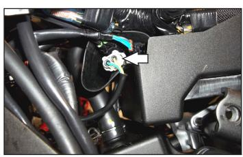
10 Plug the PC6 wiring harness in-line of the stock Crank Position Sensor connectors.
