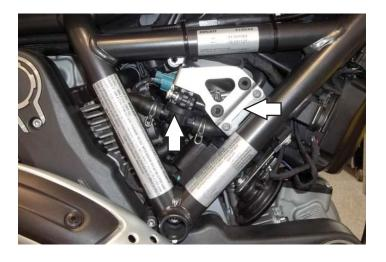
On the right side of the bike remove the PAIR valve and its bracket.
