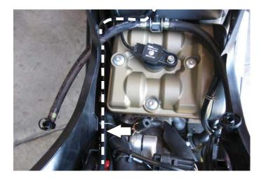
Route the PC6 harness under the subframe and go down the left side of the rear cylinder and follow the stock wiring harness to the rear fuel injector on top of the air box.
