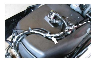
4 Continue routing the PC6 harness along the stock wiring harness to the front of the air box. Use the supplied zip ties to secure the PC6 harness to the stock harness.
