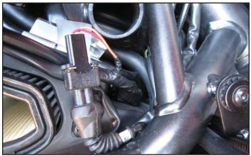
10 Plug the pair of PC6 leads with ORANGE colored wires in-line of the front fuel injector and the stock wiring harness.
