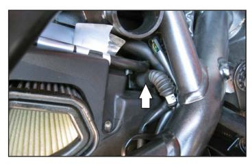
9 Unplug the stock wiring harness from the front fuel injector.
