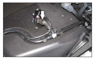
6 Plug the pair of PC6 leads with YELLOW colored wires in-line of the rear fuel injector and the stock wiring harness .
