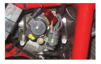
6 Using the supplied Positap, attach the single unterminated GREY wire of the PC6 to the stock ORANGE wire of the bike's TPS wiring harness.
