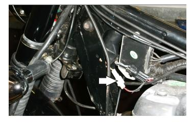
Locate and unplug the stock wiring harness from the bike's Ignition Coil, located in front of the engine head.
