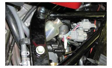
6 Unplug this connector and plug the PC6 connectors in-line.
