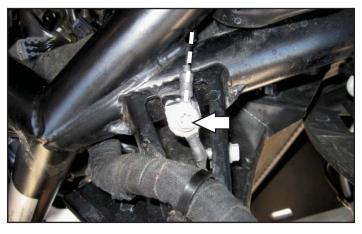
14 Attach the PC6 ground wire with the small ring lug to the stock common ground location on the right side of the frame.
