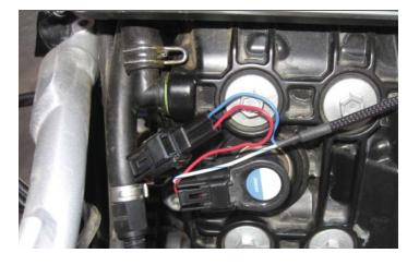
5 Plug the pair of PC6 connectors with the BLUE colored wires in-line of the Rear Ignition Coil and the stock wiring harness.
