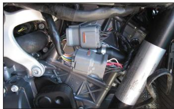
9 Locate the Front Ignition Coil and unplug the stock wiring harness from the coil.
