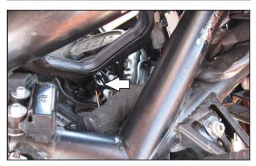
10 Plug the pair of PC6 connectors the GREEN colored wires in-line of the Front Ignition Coil and the stock wiring harness.
