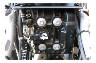
Locate the Rear Ignition Coil and unplug the stock wiring harness from the coil.
