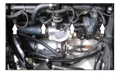
8 Plug the PC6 harness in-line of the stock wiring harness and each fuel injector.
