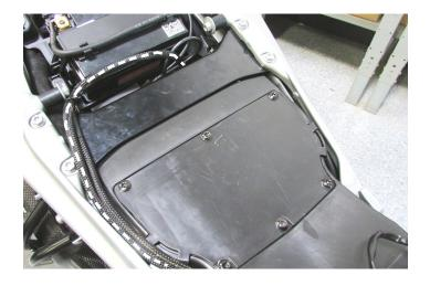
3 Route the PC6 wiring harness forward towards the engine following closely to the stock wiring harness.
