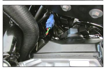
10 Plug the pair of PC6 connectors with BROWN colored wires in-line of the stock Crank Position Sensor connectors.
