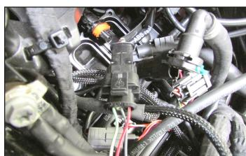
9 Unplug the Stock Crank Position Sensor connectors.
