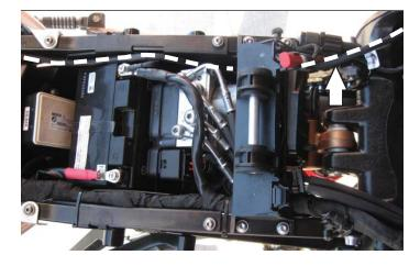
Route the PC6 harness down the left side of the bike. Route the harness underneath the fuel tank bracket and go towards the throttle bodies.
