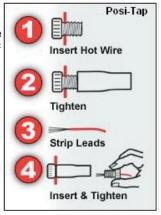
11 Using the supplied posi-tap, attach the blue wire from the PC6 to the stock purple/black wire of the gear position sensor connector.
