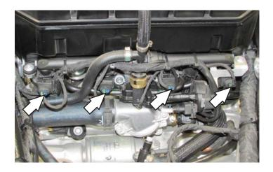
6 Plug the PC6 harness in-line of the stock wiring harness and each Fuel Injector.
