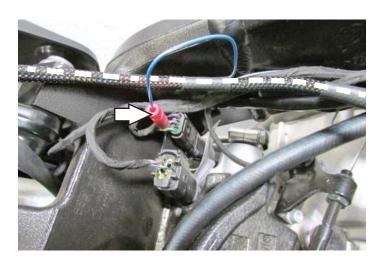
Using one of the supplied posi-taps, attach the PC6 BLUE/WHITE wire to the stock PURPLE/BLACK wire (middle wire) of the stock 3-pin Gear Position Sensor connector located on the frame of the left side of the bike.
