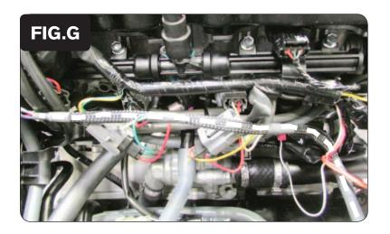
13 Plug the PCV wiring harness in-line of each Lower Primary Fuel Injector and the stock wiring harness (Fig. G).
