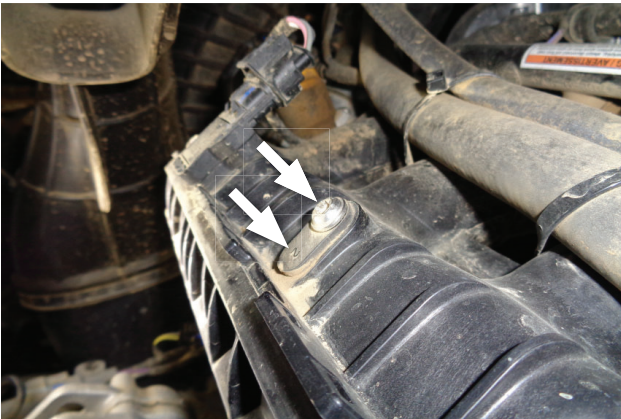
13. Remove factory screw and mount from intake. Retain screw for later use.
