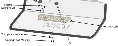
a) Install the windshield to the vehicle as shown below.
