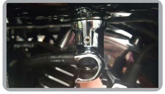
4. Tighten set screw until secure but do not over tighten.
