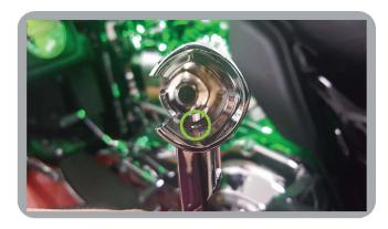
3. From bottom side of fuel fitting, push cover up and rotate to the left until in place.
