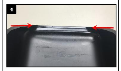
4. Test fit the new Integrated LED Taillight to underside folded lip of the fender. Make sure it is centered, then mark the position with a grease pencil for a guide. NOTE: the Integrated LED Taillight mounts on the folded lip of the fender not behind it.
