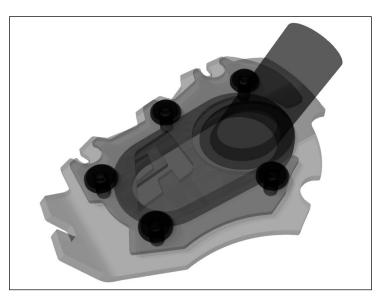
With bike on the center stand, arrange the top and bottom plates identically to how they are shown in the picture to get an idea of the fitment. Leave top plate resting on side stand. Take the (5) screws and add the washers and a small drop of thread locker to each screw. Now match up the bottom plate to the top plate and install all (5) screws with washers. Do this in the order shown in the picture.
