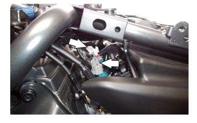
5 Unplug the stock wiring harness from each injector.
