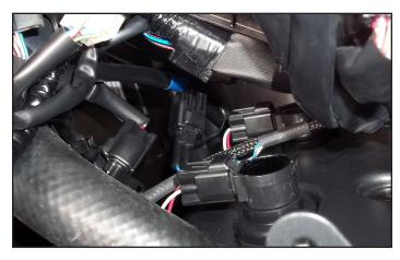
10 Plug the PCV in-line of the stock ignition coils and wiring harness.
