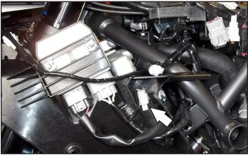
11 Unplug the stock wiring harness from the Crank Position Sensor connector.
