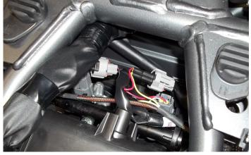
7 Unplug the stock Throttle Position Sensor (TPS) connector.
