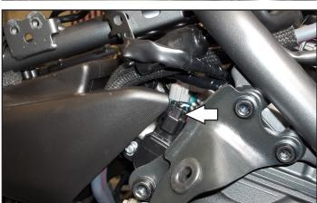
8 Plug the PCV in-line of the TPS and stock wiring harness.
